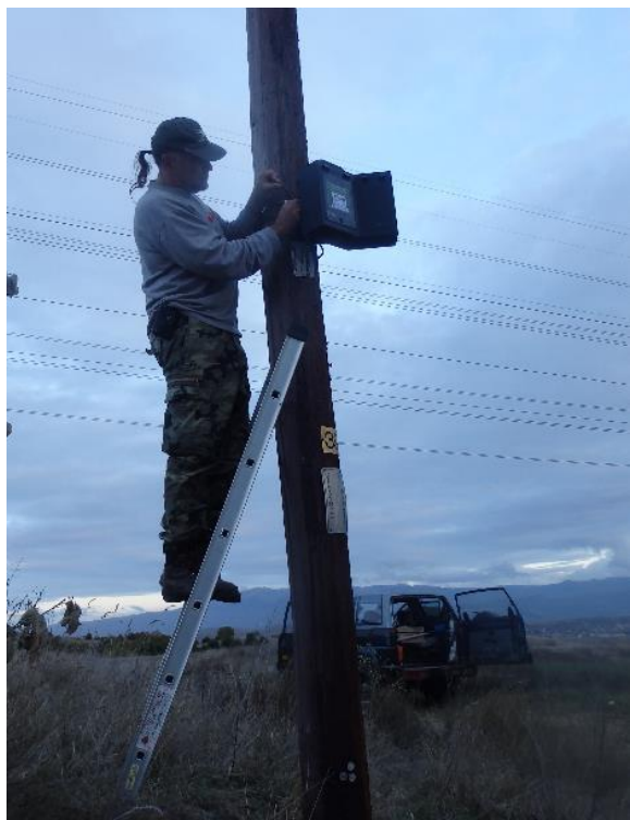
Figures 11 Mounting of Viacount II device for traffic volume and speed metering in the new highway from “Amydaio to Vevi” by using a specially constructed mounting system (above) and in the “Old highway”. When adjacent to the road power poles were available, they were also used to set the device at the appropriate height.
