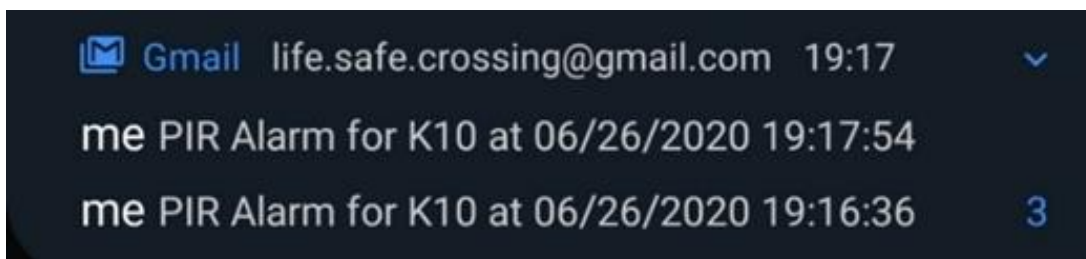
Figure 4.1.3.: Near real-time alerting @smartphone when a movement is “detected” (this implies that a snapshot (and a short video) has been taken, stored locally @camera’s SD card and uploaded automatically to COSMOTE’s cloud infrastructure)
