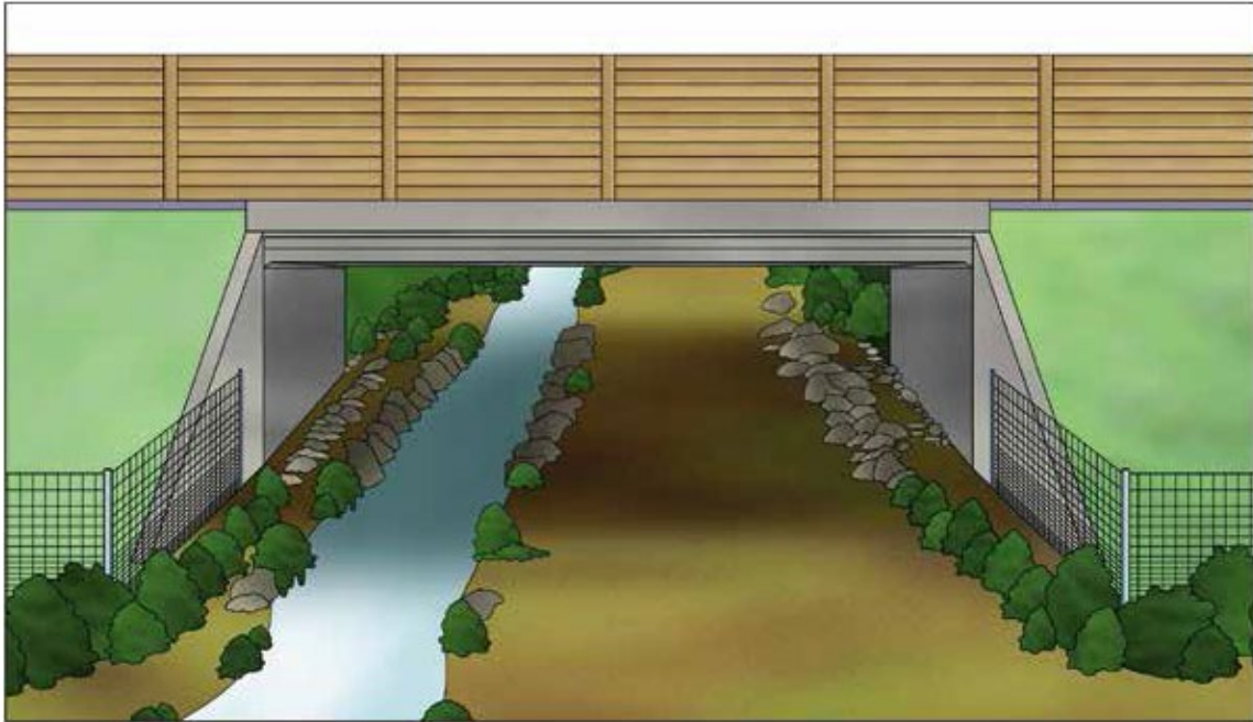
Figure 7.6. A ditch along one side of the structure leaves a large section free for use by wildlife.
