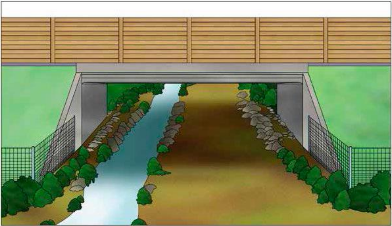
Figure 1. Drainage conduction using a ditch along on site of the underpass offers a large dry surface to be used by wildlife. Installation of opaque screens help on reducing traffic disturbances from the road or railway line above the underpass. Source: MAGRAMA 2016.
