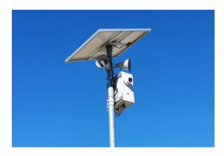
Figure 4.5. Loudspeakers to emit deterrent sounds mounted above the central unit of the AVC-PS. Photo by: LIFE SAFE-CROSSING.
