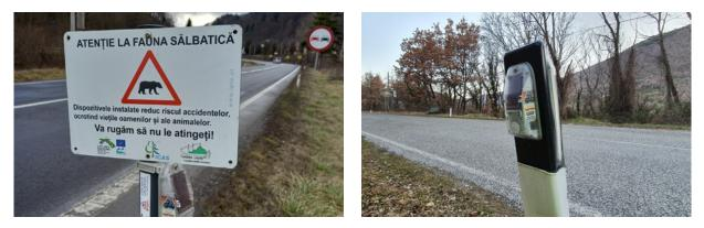
Figure 5.1. Virtual Barrier emitter units installed on road post in Spain and Italy. Photo by LIFE SAFE-CROSSING.
