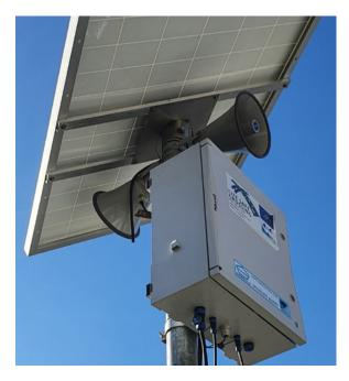
Figure 4.2. Control unit of the AVC-PS with solar panel. A. View of the interior of the box. B. General view of the control unit including electric box, solar panel, thermal camera and deterrent device. Photos by: LIFE SAFE-CROSSING.
