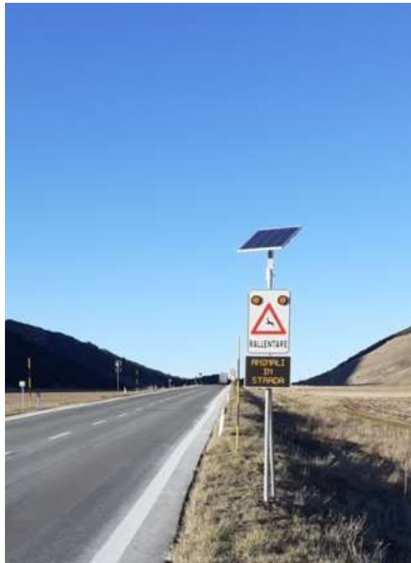
Figure 9. Flashing light panel and alphanumeric writing to alert drivers (PNM).
