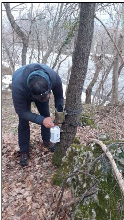
Figure 18. Camera trap and PIR sensor in PNM.
