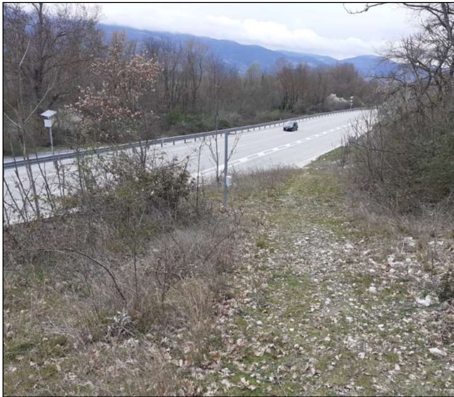
Figure 7. PIR sensor used to detect the presence of the animals approaching the road in PNM.
