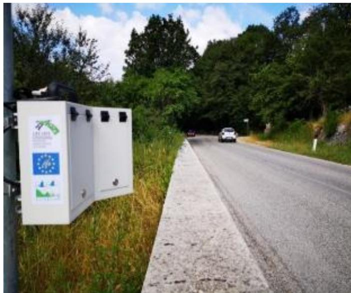
*Figure 6 Traffic counter Viacount II placed along Road\_PNALM\_B*
