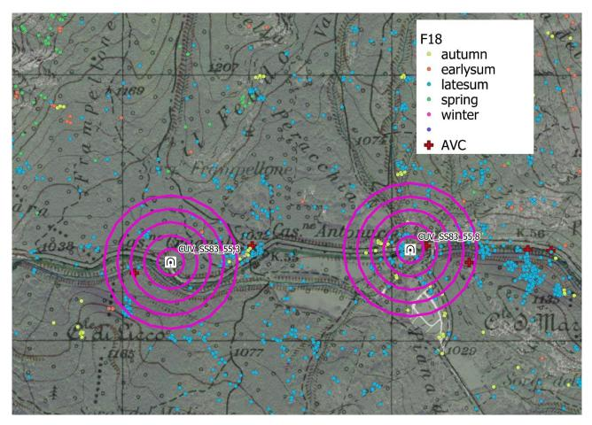
Figure 6 Location of culverts CUv\_SS83\_55+3 and CUV\_SS83\_55+8 in relation to animal vehicle collisions (red crosses) and locations of F18, a GPS collared female using the area which clearly confirm the ecological importance of this two crossing points. The circles around the culvert are buffers with an increasing radius: from 50 m around the structure to 250.
