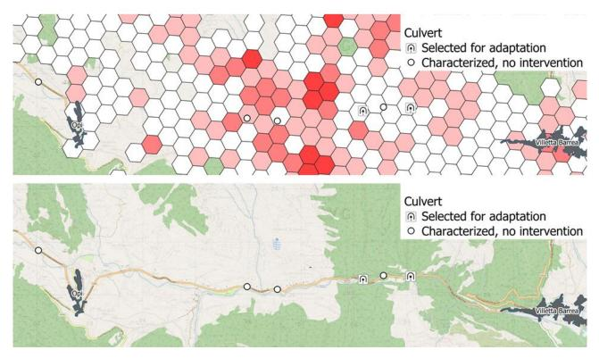
Figure 4 Transversal structures characterized along National road S.S. 83 "Marsicana", km 46–58. a) culverts characterized b) culverts in relation to the model developed in the frame of action A3: the 400 m wide hexagons indicate the amount of time spent by monitored bears in the surrounding of the road. The deepest the red the more the area is intensively used by radiocollared bears
