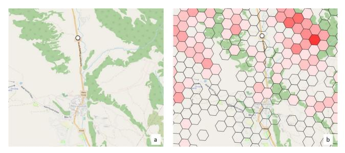
Figure 3 Transversal structures characterized along National road S.S. 83 "Marsicana", km 35 - 41 (white dots). a) culverts characterized b) culverts in relation to the model developed in the frame of action A3: the 400 m wide hexagons indicate the amount of time spent by monitored bears in the surrounding of the road. The deepest the red the more the area is intensively used by radiocollared bears
