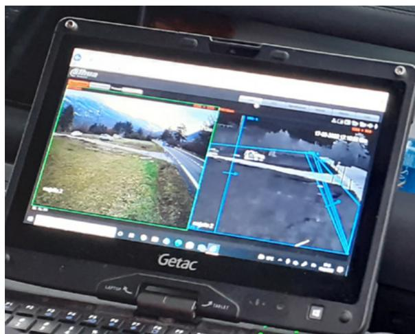
Figure 4.3. AVC-PS detection systems. A and B: PIR sensors used to detect the presence of animals approaching the road. C. Thermal camera installed in a central unit box; D. Visual and thermal images of a programmed detection area shown on a computer screen. Photos by: LIFE SAFE-CROSSING.
