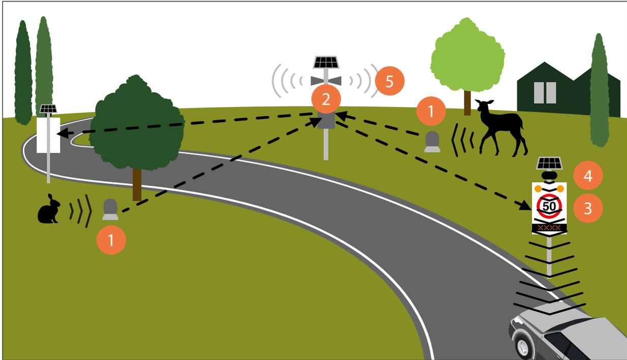
Figure 4.1. Diagram illustrating how the AVC-PS functions. 1. PIR sensors and/or thermal cameras / 2. Electronic control unit / 3. Wildlife awareness signal for drivers / 4. Radar doppler sensor / 5. Acoustic deterrent device. Source: LIFE SAFE-CROSSING.
