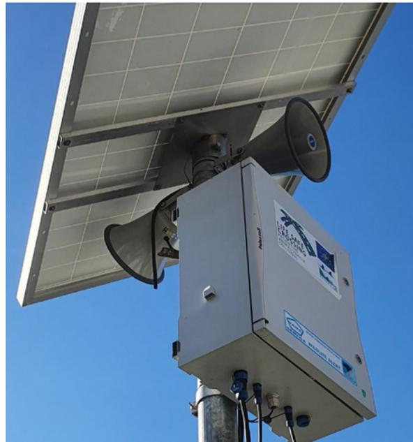
Figure 4.2. Control unit of the AVC-PS with solar panel. A. View of the interior of the box. B. General view of the control unit including electric box, solar panel, thermal camera and deterrent device. Photos by: LIFE SAFE-CROSSING.
