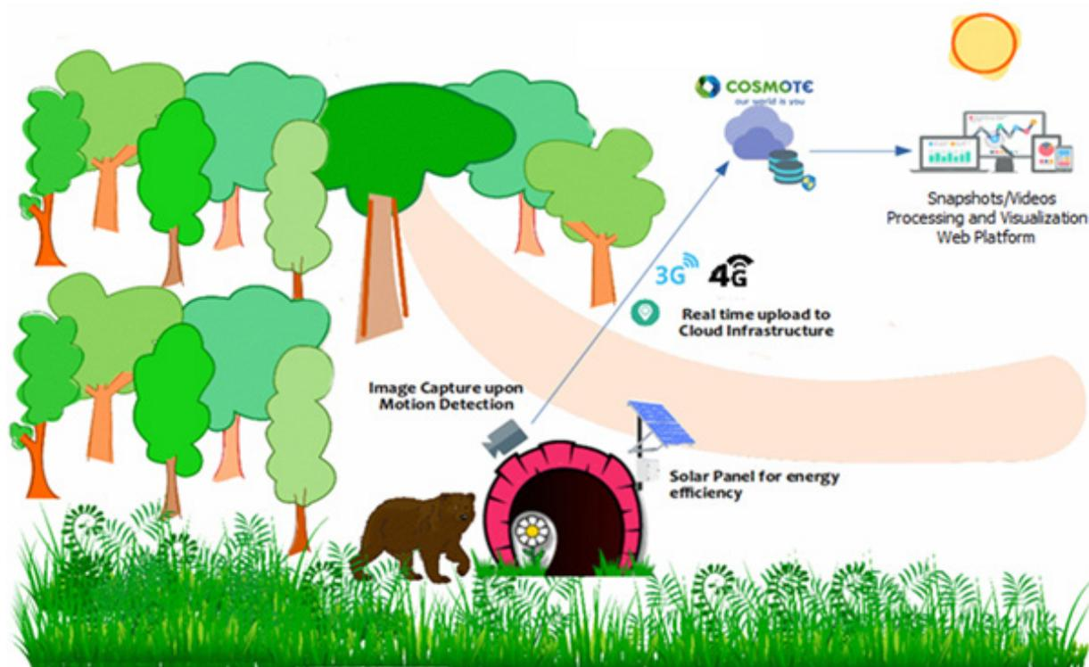
Figure 8.18. Architecture of the innovative solution applied to monitor wildlife use of crossing structures. Source: COSMOTE, LIFE SAFE-CROSSING
