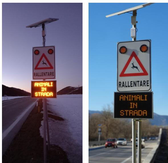
Figure 4.4. Wildlife sign connected to animal-detection systems, with flashing light and digital panels including a message to warn drivers about the presence of an animal on the road or its verges. Photos by: Minuartia. LIFE SAFE-CROSSING.
