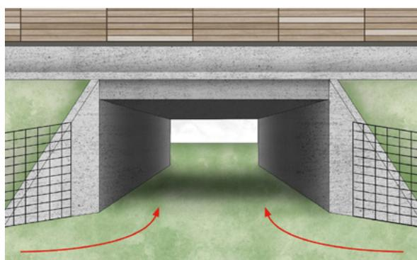
Figure 8.14. Fence fixed at the walls of the underpass funnel wildlife through the underpass and prevent access to embankments. Screen may be installed beside the road to prevent disturbance at the underpass. Photos by: Left - Egnatia Odos SA. Right - By courtesy of the IENE Biodiversity and Infrastructure online handbook.
