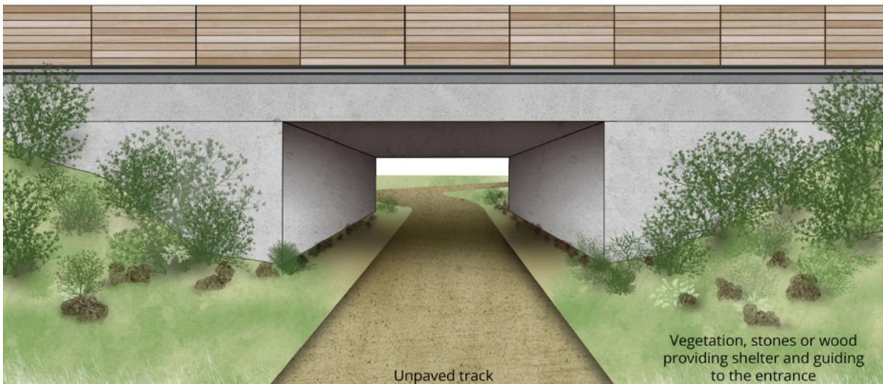
Figure 8.12. Vegetation distribution and fencing must funnel wildlife to the entrance of wildlife passages and provide refuges at both sides of the structures. Wood screens may be installed to reduce disturbance from traffic. Source: by courtesy of the IENE Biodiversity and Infrastructure online handbook.
