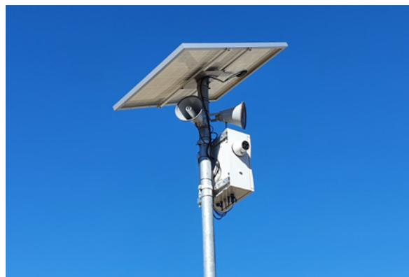
Figure 4.5. Loudspeakers to emit deterrent sounds mounted above the central unit of the AVC-PS. Photo by: LIFE SAFE-CROSSING.
