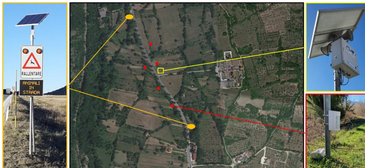
Figure 4.7. Position of the different components of an AVC-PS. Example from Maiella National Park. Road SS 17 in Pettorano, including 5 sensors and 1 thermal camera. Photos by: Maiella National Park.
