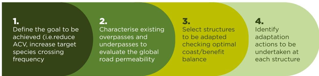
Fig 8.2. Steps for upgrading existing overpasses and underpasses to enhance their use by wildlife achieving an optimal cost/benefit balance.
